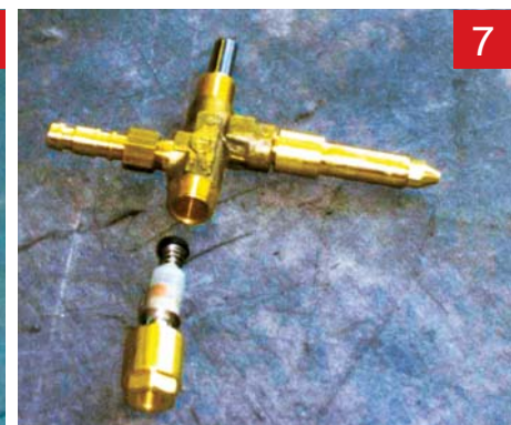
Carefully take out the injector 小心翼翼地取出喷射器
