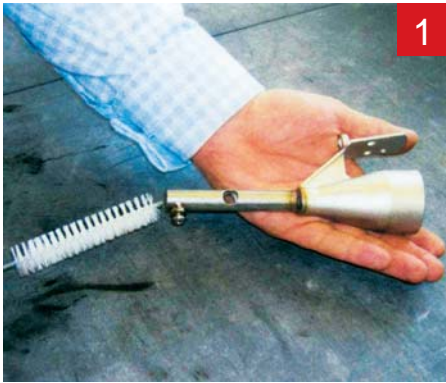
Disassemble the Venturi from the body 通气管从育雏器主身拆卸
